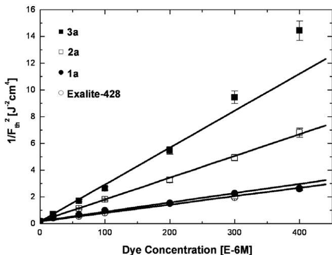
Fig. 3. Plots of  $1/F_{th}$  against the dye concentration in PMMA thin films. Exalite-428 (open circles), **1a** (closed circles), **2a** (open square) and **3a** (closed square). The data are fitted to straight lines by the least square method by assuming that the intercepts are constant. (see the text).
