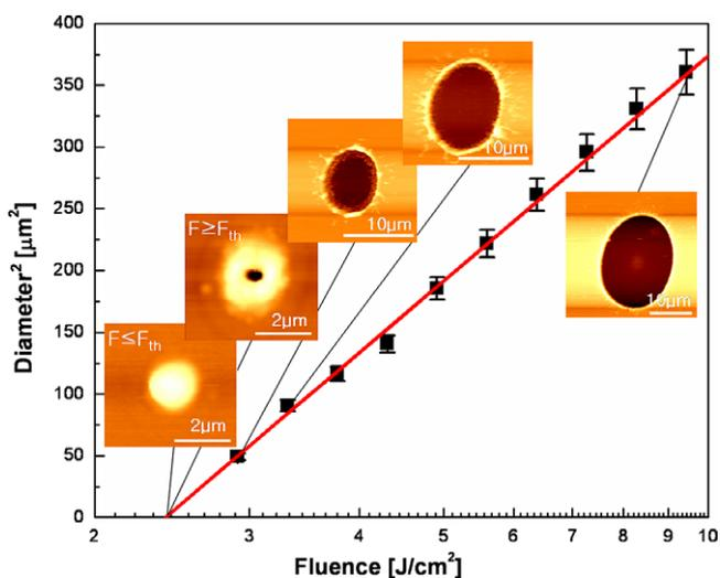
Fig. 2. Squared diameter  $D^2$  of the ablated area of pure PMMA thin films as a function of laser fluence. The insets show the changes in the morphology of the film surface at five different laser fluences. The film thickness is 250 nm.
